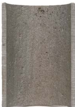
Treated with Acid and OxiFlo ® Oxidizer All biofilm and scale removed.
