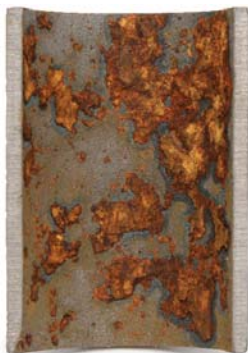
Treated with Acid Only Scale protected under biofilm not removed.
