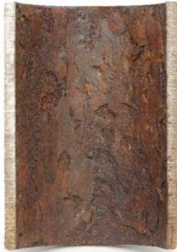
Untreated Completely coated with scale & biofilm.
